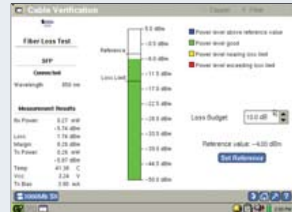
Ensure optical power limits are within specification
